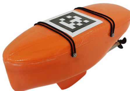
Figure 5 A 3D printed USV platform designed for indoor swarm research [9].
