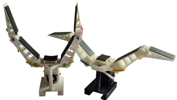
Fig. 2. The initial prosthetic hands that were used to test tendon routing and rigidity when the hand is assembled. On the right is the first iteration and on the left is the second that aimed at reducing the weight of the overall assembly.
