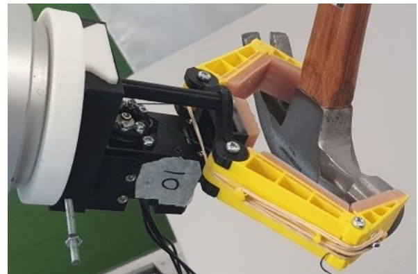
Fig. 10. The proposed highly under-actuated prosthesis gripping a hammer in a pinch grip around the head.
